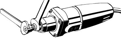
Follow the same procedure to change the collet, except collet nut must be completely unscrewed in order for the collet to be changed.
