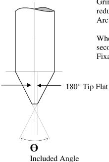
Grinding a tip flat on electrodes increases arc stability and reduces arc wander. Many TIG, Automated TIG, and Plasma Arc Welding applications call for precision tip flat.
