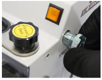
By loosening the M6 Locking Nut, the depth of the set screw can be adjusted. Please refer to the following table for adjusting the depth according to the diameter of the electrode and the desired angle.
