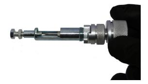
Use the electrode set gauge for identical grind angles on every electrode. Insert the Collet Chuck Assembly with the tungsten electrode into the Electrode Set Gauge so that the notched portion of the assembly fits completely into the notched portion of the receptacle and the tungsten electrode is making contact with the set gauge.
