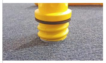
• Now test fit your divider again, remove more if necessary. You want to achieve a mild press fit. When there is enough clearance start pressing the divider into place. When the diver is <sup>1</sup>/<sub>3</sub> to <sup>1</sup>/<sub>2</sub> way inserted turn the assembly upside down then lightly press or tap it in place.
